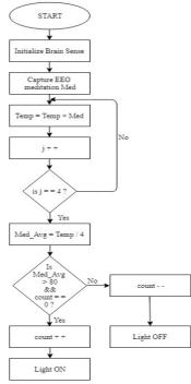
Fig. 1. Design flow for mode I
